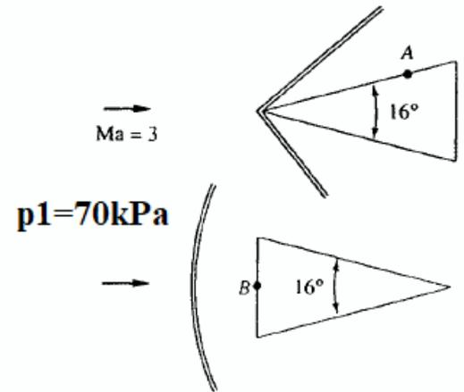
(b) A normal shock forms, and  $p_B = p_{o2}$  inside the shock. Given  $p_{o1} = p_1/0.0272 = \mathbf{2573.529 \text{ kPa}}$
