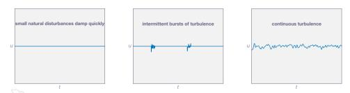
Fluctuations in the fully turbulent flow velocity signal:
