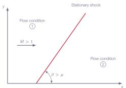
Significant changes of flow properties from 1 to 2
