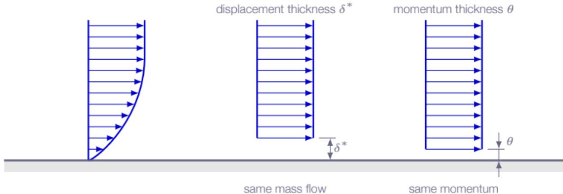
*"The presence of a boundary layer will result in a small but finite displacement of the flow streamlines"*
