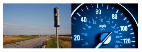
Eulerian Frame of Reference fluid properties as function of position and time Lagrangian Frame of Reference follows a system in time and space
