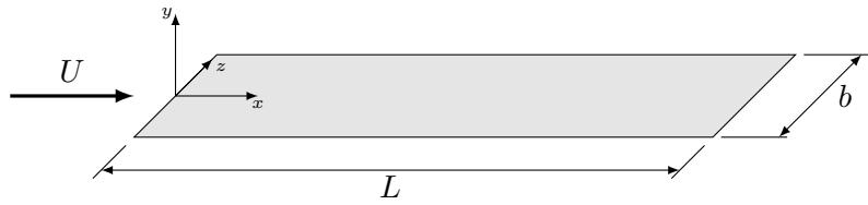
A flat plate is placed in a wind tunnel as part of an experimental setup. The boundary layer that builds up over the flat plate surface leads to a drag force that must be handled by the fastening devices. The flat plate will also be used for a similar experiment in a water tunnel, where the drag force will be greater. Flow and fluid properties are given in the table below (use the same temperature and velocity for the water tunnel experiment and the wind tunnel experiment)
