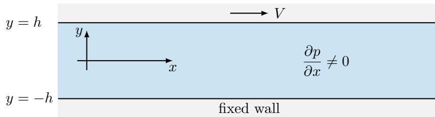
The fluid flow between two parallel plates is driven by a moving boundary (the upper plate is moving at a constant velocity  $V$  in the positive  $x$ -direction) and a non-zero pressure gradient. The fluid is incompressible and the flow can be assumed to be steady and fully developed. There is no flow in the  $z$ -direction and gravity can be neglected.
