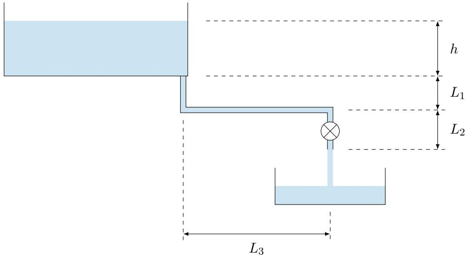
Water @ 20°C is drained from a tank through a 0.1 m diameter ( $D$ ) pipe attached to the bottom of the tank (see figure above). The pipe has two 90° bends, each with a loss coefficient of  $K = 0.23$  and a valve with a loss coefficient of  $K = 2.0$ . The tank can be assumed to be very large which implies that the water level ( $h$ ) can be approximated to be constant. The pipe lengths  $L_1 - L_3$  are given in the table below.
