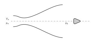
A model of a re-entry vehicle (a very blunt object) is to be tested in a supersonic wind tunnel at a freestream Mach number of 4.0. The test section (where the model is placed) is located inside of a vaccum tank and during the test, the pressure in the tank, the pressure downstream of the nozzle exit  $(p_b)$ , is reduced to 10% of the atmospheric pressure. The nozzle-exit cross-section area is 1.0  $m^2$
