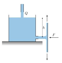
A water tank with the diameter  $D = 5.0 \ m$  is constantly filled from above such that the water level in the tank is constant at  $h = 2.0 \ m$  above the discharge orifice located in the lower part of the tank. The diemater of the discharge orifice is  $d = 5.0 \ cm$ . The temperature of the water in the tank is  $20^{\circ}C$ . The water jet emanating from the orifice hits a plate oriented normal to the jet flow.
