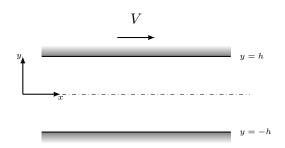
A lubrication film (SAE 30W oil at a temperature of  $20^{\circ}C$ ) flows between two parallel plates separated a distance of  $2h = 2.0 \ mm$ . The upper plate moves to the right at a constant velocity of  $V = 0.5 \ m/s$  and the lower plate is fixed. The flow between the plates is driven by the moving surface but is also affected by the presence of a constant pressure gradient. Thus, the flow is a combined Couette-Poiseuille flow. The flow can be assumed to be fully developed.
