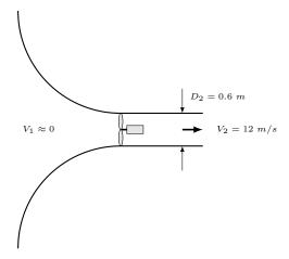
An axial-flow fan installed in an air ventilation system is driven by an electric motor marked 0.4 kW. The flow velocity in the air intake ahead of the fan can be assumed to be zero and after the fan, the fluid velocity is 12.0 m/s. The duct in which the fan is installed has the diameter D = 0.6m.
