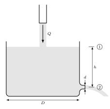
(a) Tank problems are often solved assuming that the fluid velocity at the surface is zero. Obviously, the fluid velocity cannot be zero, but it is often a good assumption. The assumption gets better as the ratio d/D decreases. Calculate the ratio d/D such that the error is 0.01%. (6p.)
