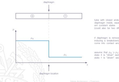
diaphragm inside, separating two different constant states (could also be two different gases)
