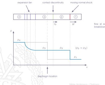
flow at some time after diaphragm breakdown
