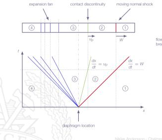
flow at some time after diaphragm breakdown
