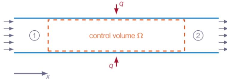
1D pipe flow with heat addition:
