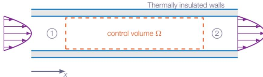
1D pipe flow with friction:
