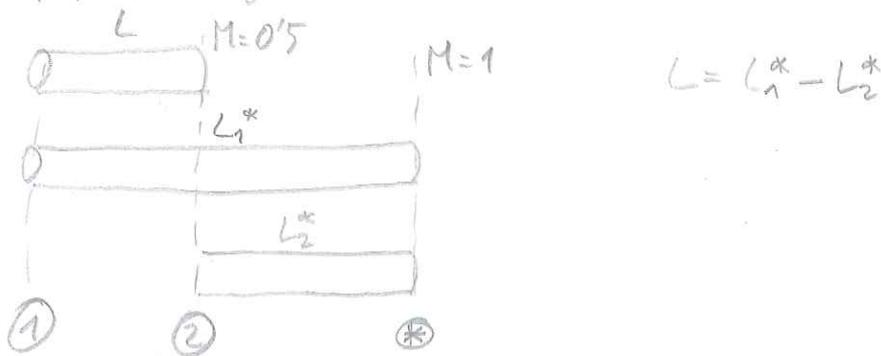
We start by assuming the inlet is condition 2 so that we can find  $L_2^*$ . Using table A.4 with  $M_2 = 0.5$
