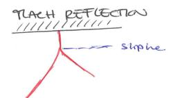
A REGIMAR REFLECTION WILL ACCUM IF PADARIE IN THE EXAMPLE SHOWN ABOVE THE FIRST SHORL DEFLECTS THE FILM AN ANGLE & AND AT THE FLOW MALL THE FLOW MUST BE DEFLECTED BACK IF & < & max AT 91=M2 WE WILL GET A REGIMAR REFLECTION . IF & > & me WILL INTEAD GET & MACH REFLECTION
