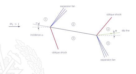
It seems that the angle of the flow downstream of the flat plate would be different than the angle of the flow upstream of the plate. Can that really be correct?!
