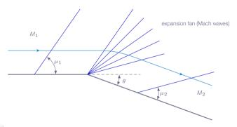
$M_2 > M_1$  (the flow accelerates through the expansion fan)
