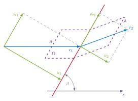
Two-dimensional steady-state flow Control volume aligned with flow stream lines
