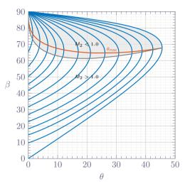
**Note!** In Chapter 3 we learned that the Mach number always reduces to subsonic values behind a shock. This is true for normal shocks (shocks that are normal to the flow direction). It is also true for oblique shocks if looking in the shock-normal direction.
